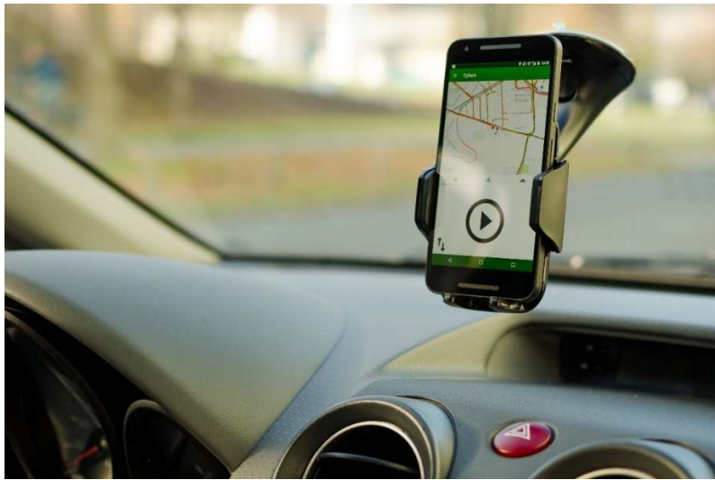
Fig. 2: Smartphones are mounted on the windshields of vehicles and used as mobile sensor units. Image credit: Cyface GmbH.
