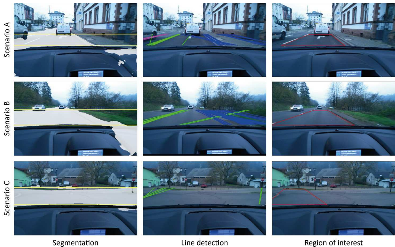
Fig. 4: Automated ROI detection. We combine information from line detection using the Hough transform (left) and a semantic scene segmentation approach based on Deep Learning that is able to detect the parts of the image pertaining to the street or road (middle) to automatically determine a quadrilateral region of interest for each image. (Own source)
