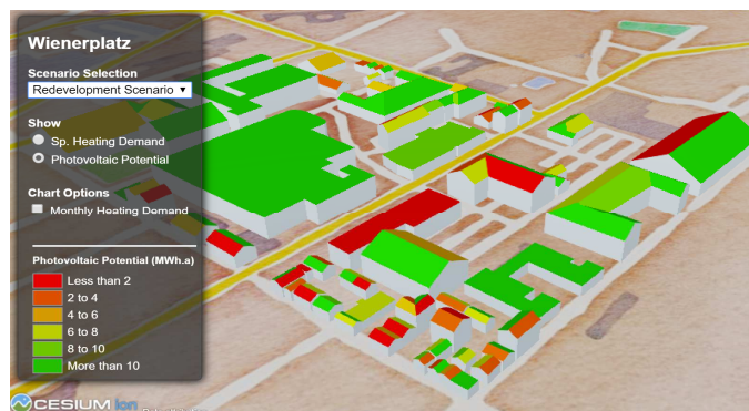
Fig. 16: SimStadt's photovoltaic potential analysis of roof surfaces visualised on cesium globe
