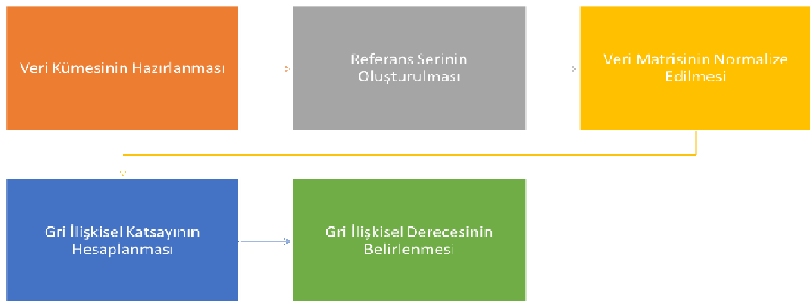
Fig.1: Process of calculation for Gray Relational Analysis (GRA)
